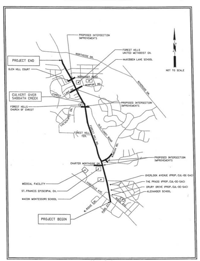
intersection indicates that this intersection is a logical terminus for the four-lane typical section. The proposed typical section of Forest Hill Road north of this intersection would be a three lane urban section.
