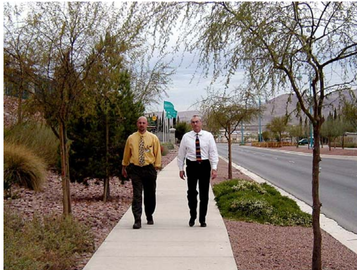
Detached sidewalk with planted buffer strip This provides the pedestrian with a secure area to move through the corridor. Note the width of the sidewalk that allows pedestrians to walk comfortably side by side.
